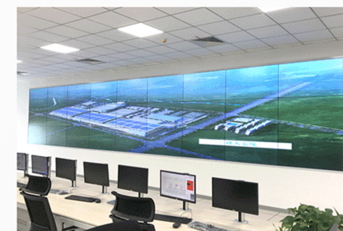
某地区工厂监控室 Factory monitoring room in a region 3x9 55寸拼接 3x9 55 inch video wall
