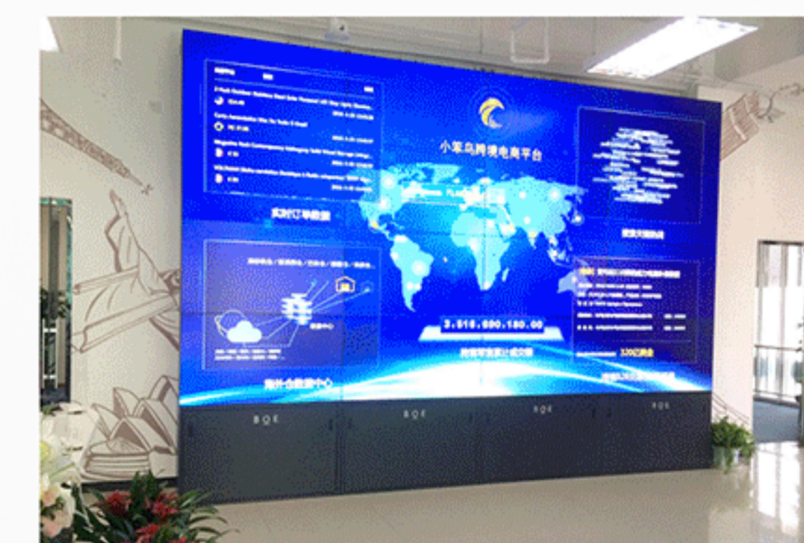
某跨境电商平台 A building, conference room 4x4 55寸拼接 4x4 55 inch video wall
